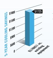
SEER stands for "Seasonal Energy Efficiency Ratio" and is a measure of the cooling efficiency of air conditioners. The higher the SEER, the greater your energy savings. Typical SEER ratings start at 13.00, but the EL16XC1 carries ratings as high as 17.00.
